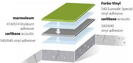
acoustic with a water-based acrylic adhesive i.e 540 Eurosafe Special approx. 150-200g/m<sup>2</sup>.
